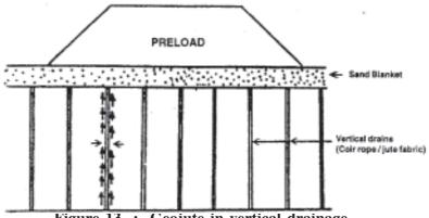
Figure 13: Geojute in vertical drainage
