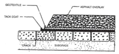
Figure 4. Geotextile as pavement overlay for treatment of cracks in airport runway.
