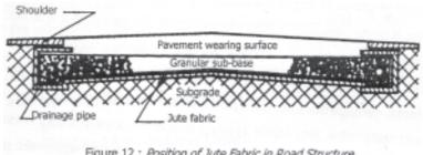
Figure 12: Position of Jute Fabric in Road Structure
