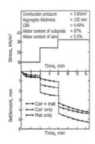
Figure 2: Short Time Rutting Test
