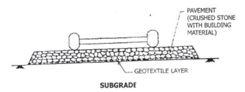
Figure 1 : Geotextile in temporary roads.
