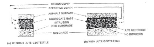
Figure 9: Pavement with Jute Geotextile
