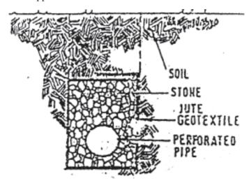
Fig. 8 : JUTE INTERCEPTOR DRAIN (after Ramaswamy et al. 1992)
