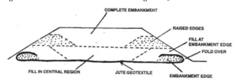
Figure 11: Geojute in embankment construction
