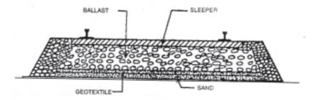
Figure 5: Geotextile in strengthening railway track.
