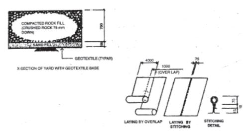
Figure 2: Geotextile in fabrication yard near Haldia Port.
