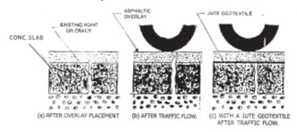
Figure 10: Control of refractive cracking with Jute Geotextile
