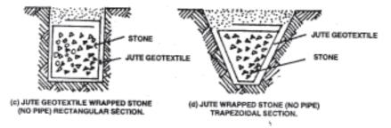
Figure 12: Jute Geotextile in trench drains
