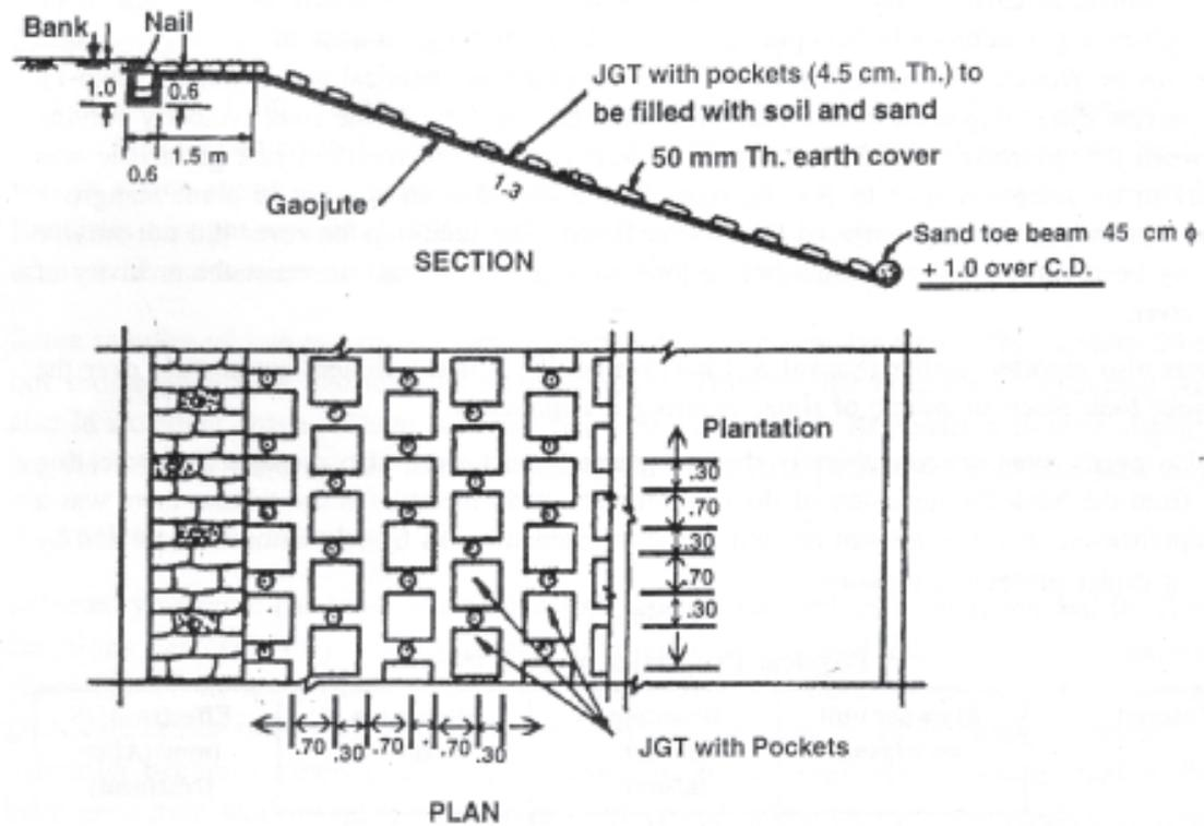
Figure 4 : Typical Sectional Elevation & Plan for bank protection & mangrove plantation (JGT with pocket type)
