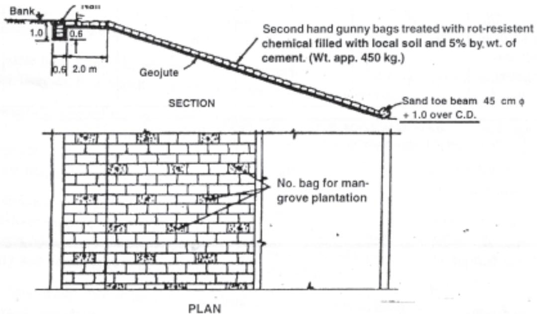
Figure 5 : Typical Sectional Elevation & Plan for bank protection & mangrove plantation (Gunny bag type)
