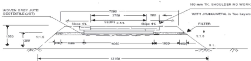
Fig. 6 : Typical cross-section of the road
