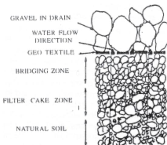
Fig. 1. Graded filter developed within the soil adjacent to the geotextils
