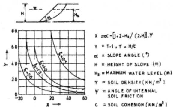
Fig. 4. Slope stability as a function of slope geometry and soil shear strength
