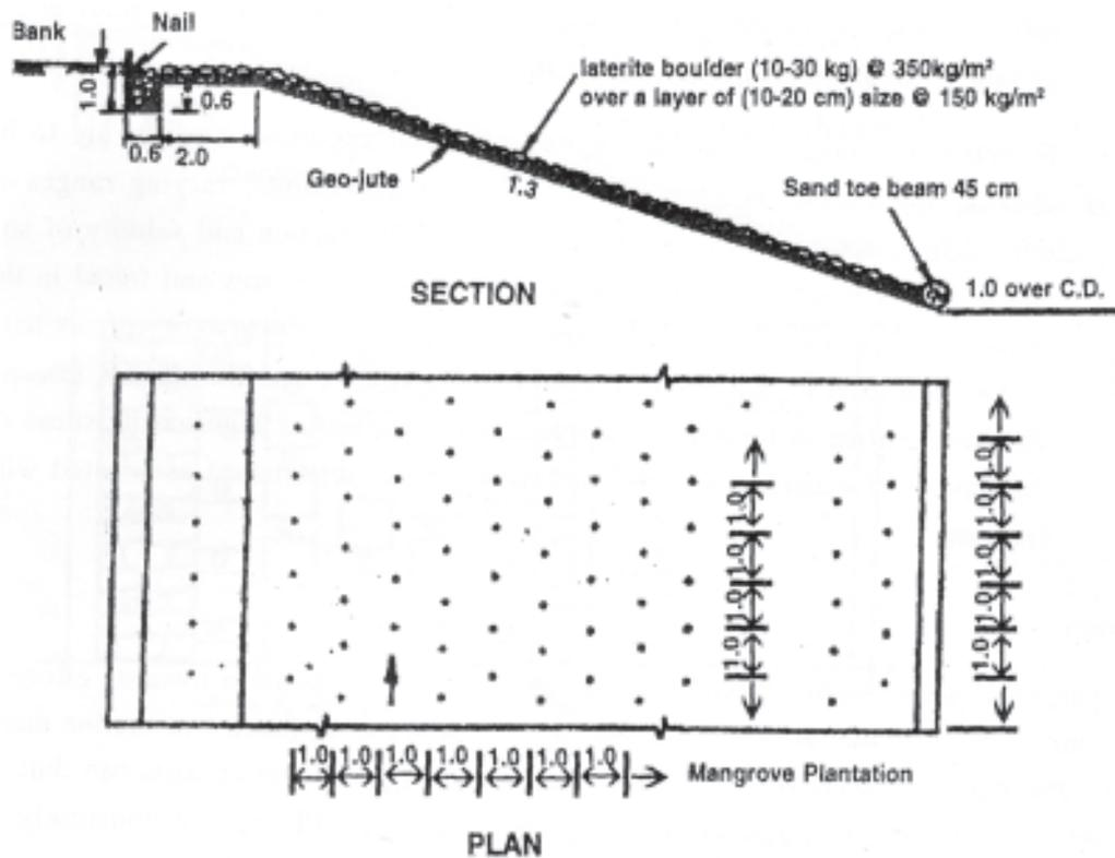
Figure 3 : Typical Sectional Elevation & Plan for bank protection & mangrove plantation (Boulder type)
