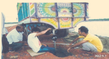
Fig: Conducting field CBR test during 1 st monitoring
