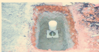
Fig: Performing Field density test during 2 nd monitoring
