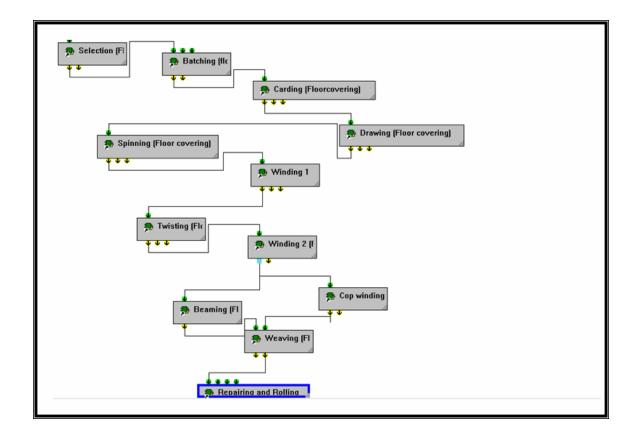
Modelling for Gate to Gate Phase of Jute Geotextiles (Woven)
